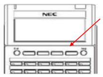
**Soft keys** are located below the display screen. Each of the 4 buttons will correspond with the feature name shown directly above it in the display screen. They will change based on the status of the phone (idle, off hook, on a call, etc.)
